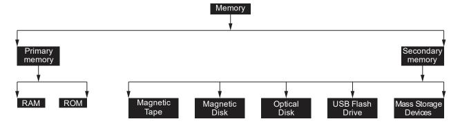
Fig: Classification of Primary memory and secondary memory
