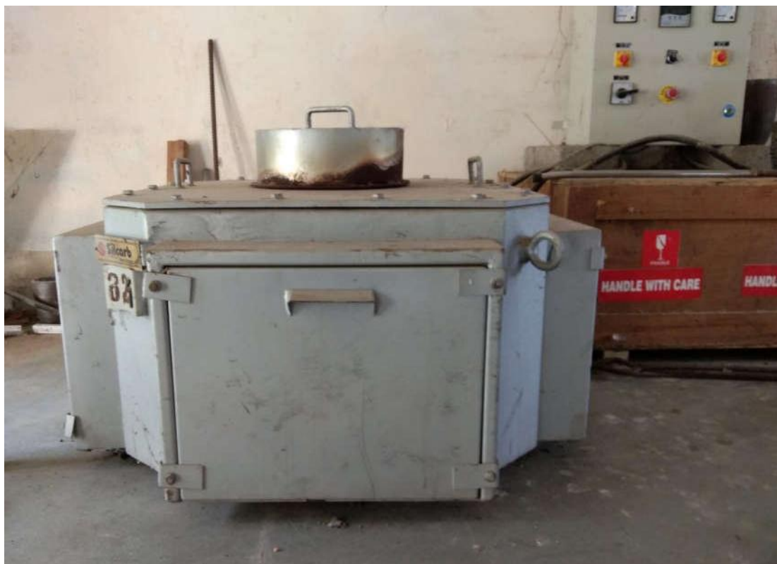
Fig.1 Electric resistance furnace with controll unit.
