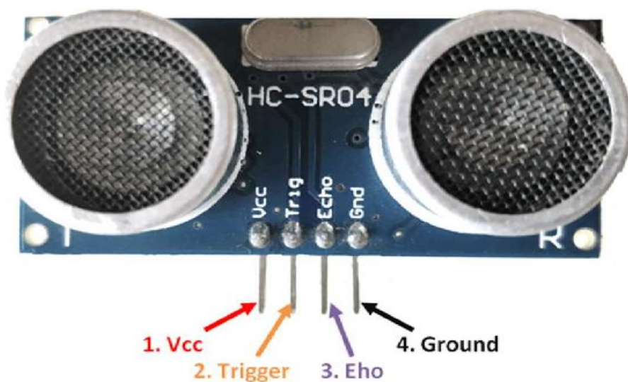
Figure 3. Pin diagram of Ultrasonic Sensor
