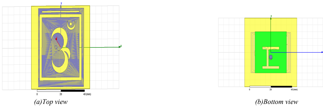
Fig 1: Microstrip patch antenna with Partial & defected Ground structure
