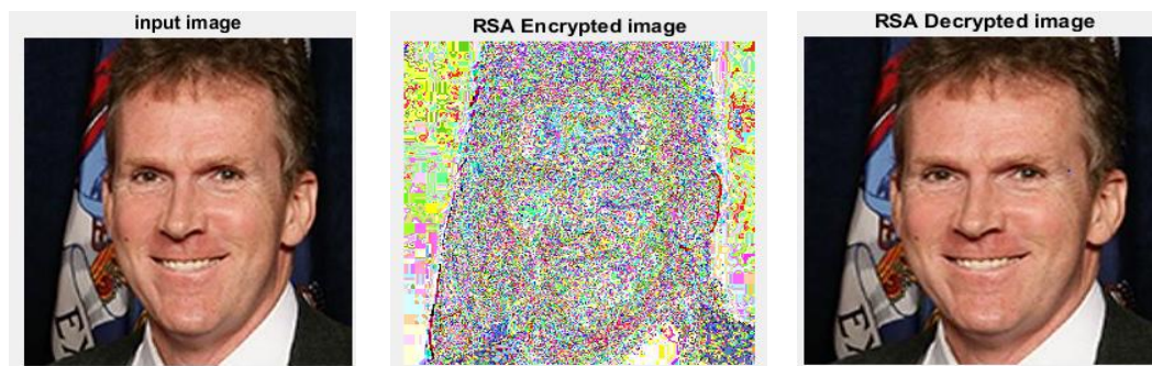
Fig. 4: Example of RSA encryption and decryption; p=13 , q=31 , n=403 , \phi_n=360 , e=7 , d=103
