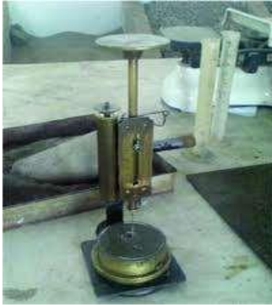
Fig5.2 Vicat Apparatus to find initial setting time
