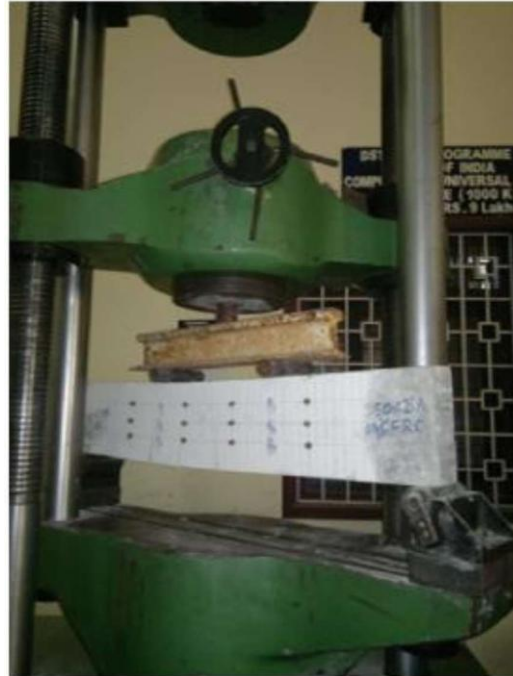
Flexural test on beam with BGC3 mix
