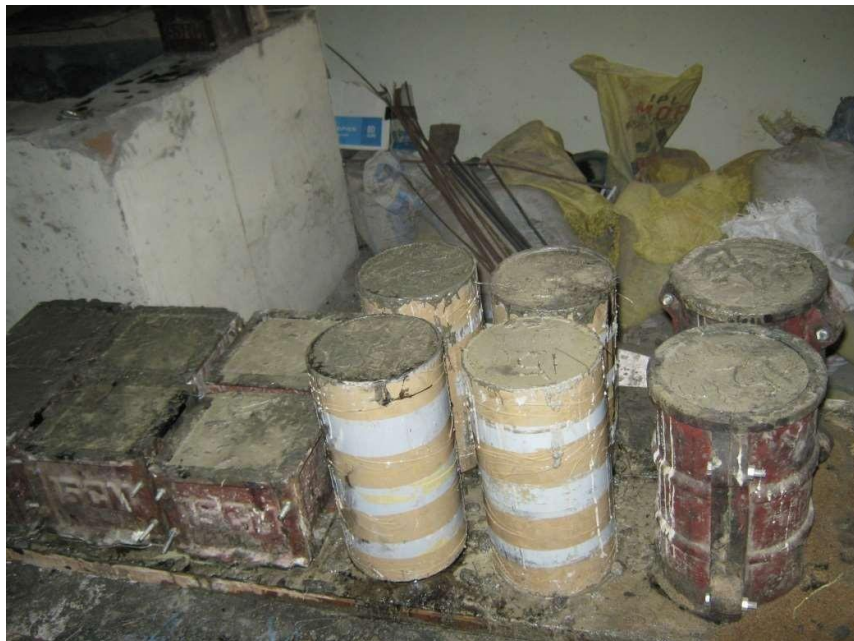
Fig 7.7 Specimen after Casting
