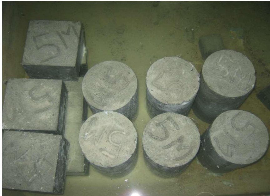
Fig 7.8 Specimen in Curing Tank for Curing
