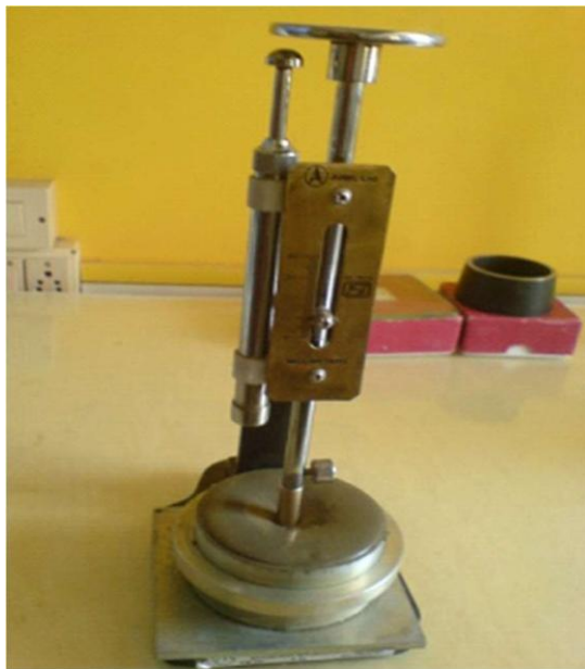
Fig5.1 Standard Consistency Test
