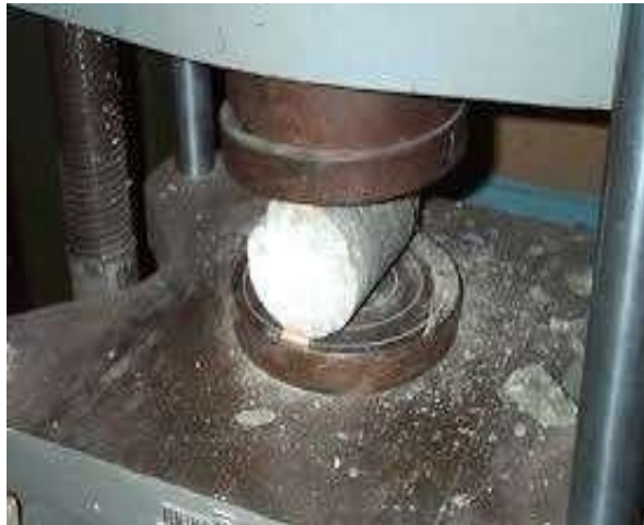
Fig 7.2 Split Tensile Test
