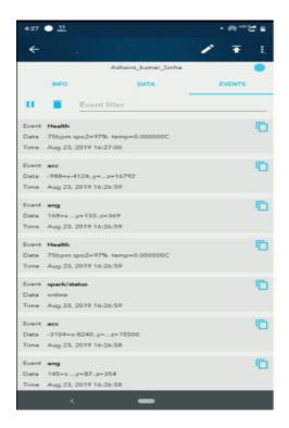
To get the data from the device cloud Open the console and copy the URL and paste it in any browser then it will show data with event name. This data can be accessed from anywhere over internet no matter how far you are from the device and the live data of the sensors can also be accessed from Particle App.
