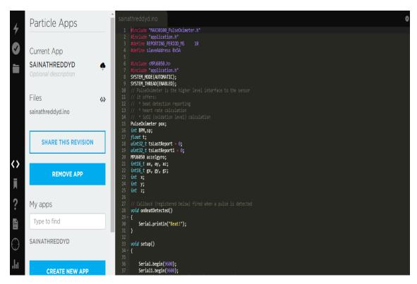
After connecting the system with the Wi-Fi router that is our connection status is shown in the Particle web IDE will show online. Now open the Arduino IDE in your PC and connect the Bluetooth HC-05 to your PC. After checking the Bluetooth Com PORT Number and change the port to that port . Now open the Serial port where you can see the live sensor data of the athlete.
