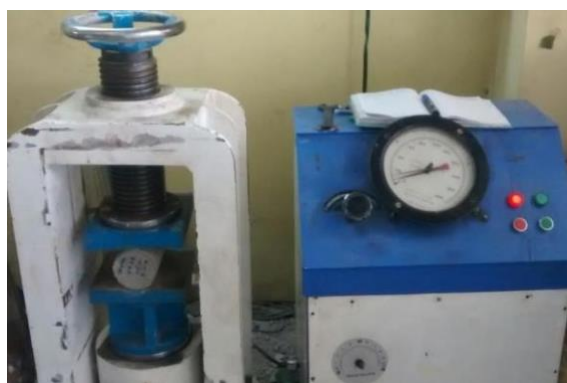
Fig -2: Split tensile Strength – Experimental set up
