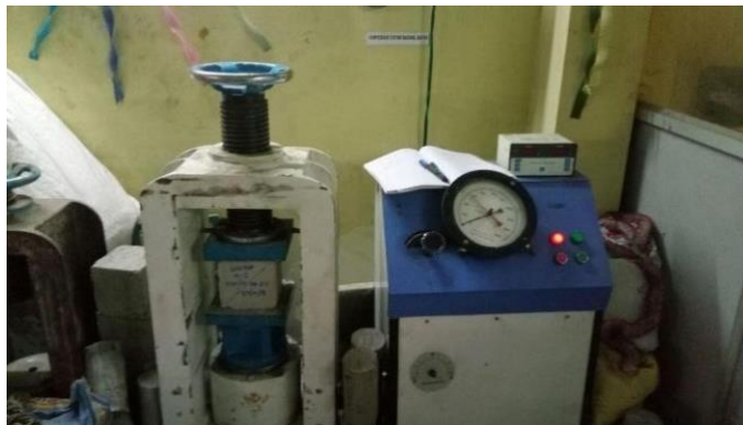
Fig -1: Cube Compressive Strength – Experimental set up
