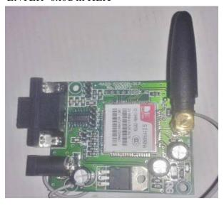
The SIM900 is a complete Quadband GSM/GPRS
