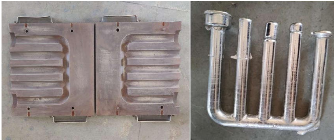
Fig.2 (a) Metallic Die (b) Casting after solidification
