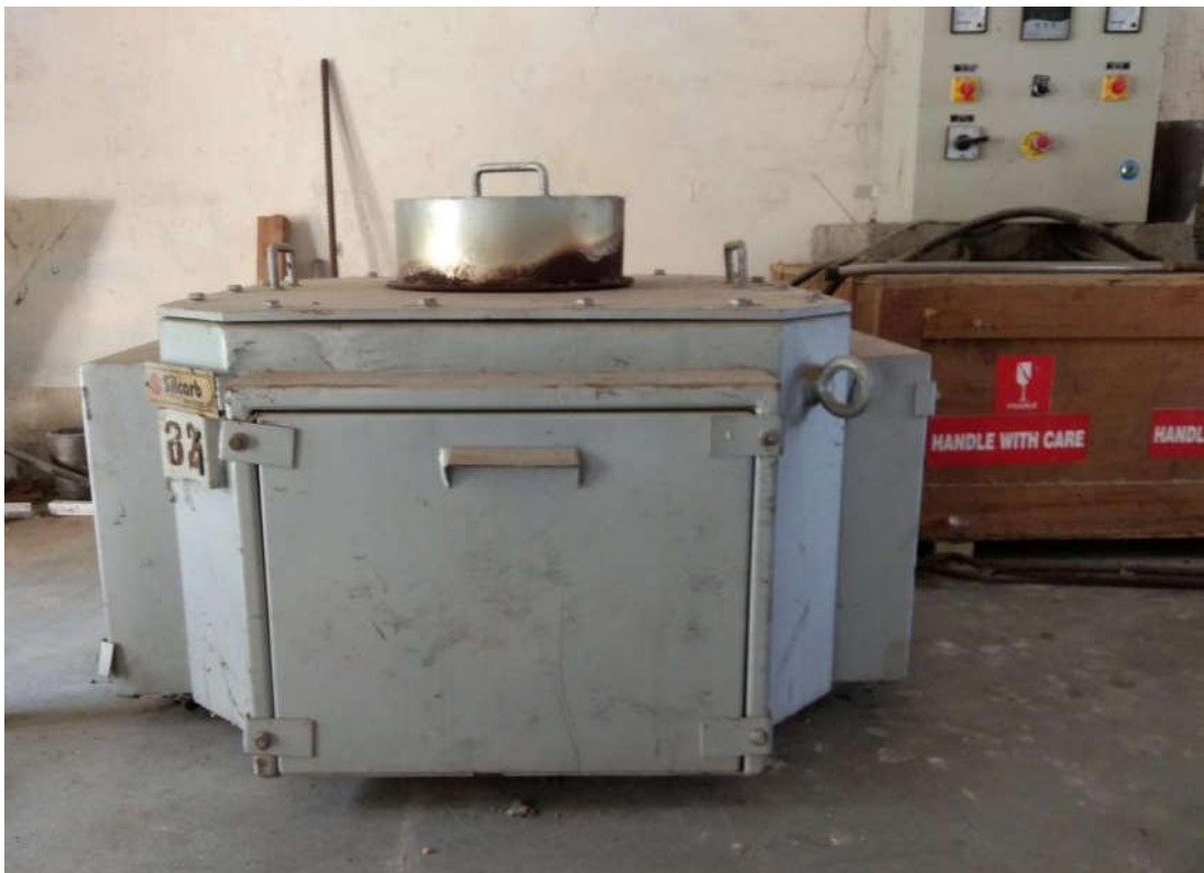
Fig.1 Electric resistance furnace with controll unit.
