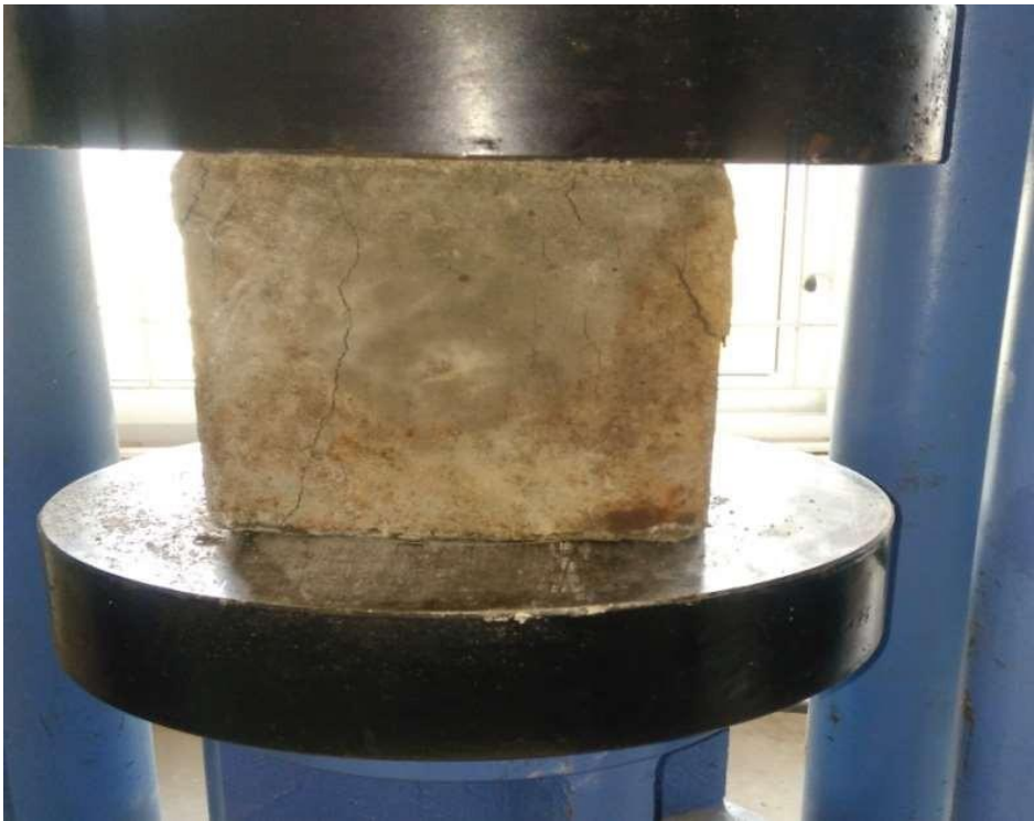
FIG 5.4 COMPRESSIVE STRENGTH TEST
