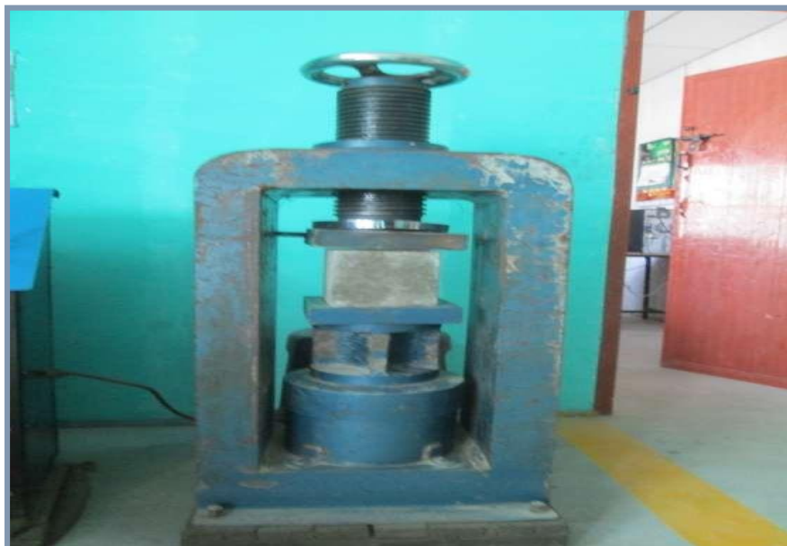
FIG 5.3 CUBE FOR COMPRESSIVE TEST
