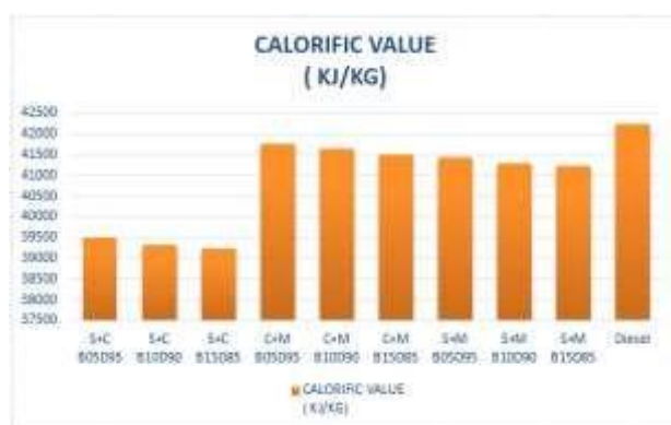
Figure 6 Calorific values of different Biodiesel blends.
