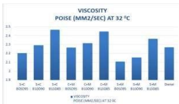
Figure 2 Viscosity of different Biodiesel blends.
