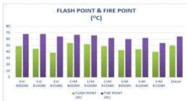
Figure 4 Flash point and Fire point of different Biodiesel blends.
