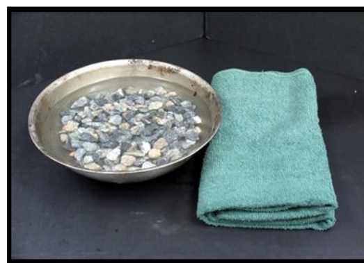
Fig 3 -Water absorption of coarse aggregate
