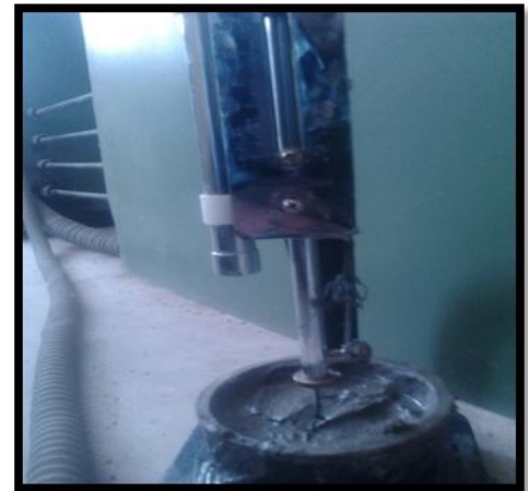
Fig 4- Initial setting time test
